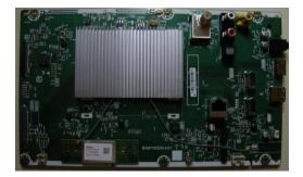
When replacing the Digital Main, the antenna cable must be removed from the defective board and installed on the new board.
