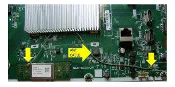
Failure to move the cable will result in the lack of range for the microphone.
